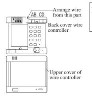
Note: When connecting wire, please keep a certain distance between signal wire and electric wire. (over 10mm)
